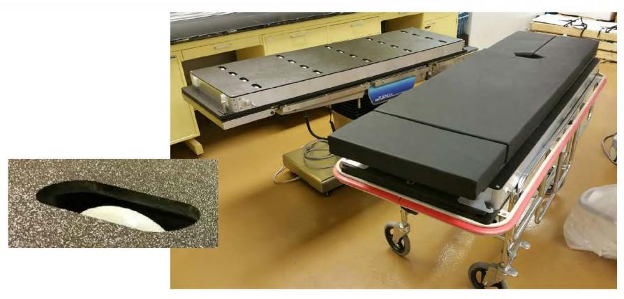
The prototype system mounted on an OR table and gurney in the ECORE Bio-Skills Lab. Here the "patient" is on the gurney and the rollers are retracted on both units
