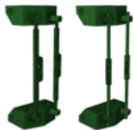
Figure 1. ASTM F1717 constructs (Low cost construct(left)-Traditional Growth Rod(right))
